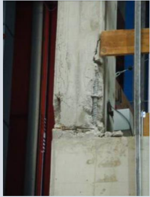
Failure of the lap splice joint N frame
