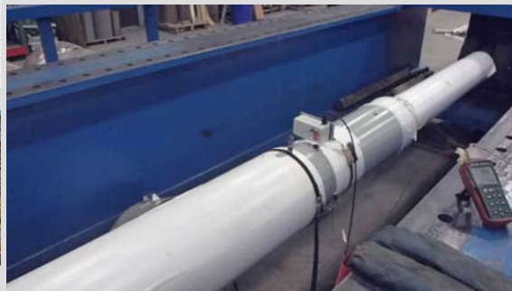
WASHINGTON HOSPITAL PROTOTYPE TESTING PEAK FORCE=2050kN, DISPLACEMENT=500mm, VELOCITY=2400mm/sec TAYLOR DEVICES TESTING MACHINE, MAY 2013
