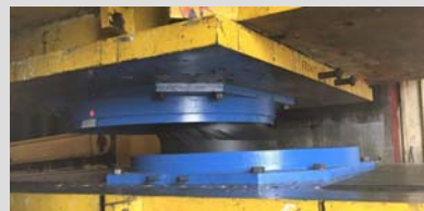
2059 TRIPLE FP PRODUCTION ISOLATORS TESTED, 2017
