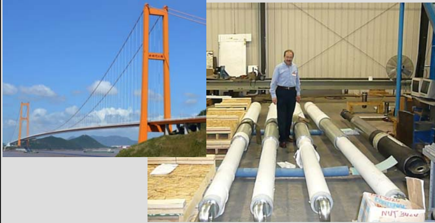
XIHOUMEN BRIDGE, CHINA 8.8m LONG WHEN EXTENDED +/-1.2m DISPLACEMENT CAPACITY 1000kN RATED LOAD CAPACITY
