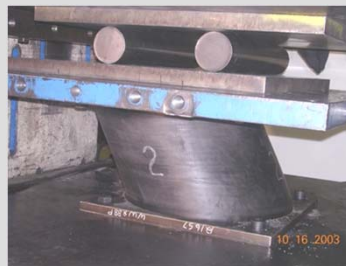
LEAD RUBBER BEARING DYNAMIC TESTING AT VELOCITY OF 250mm/sec, LOAD=1500kN
