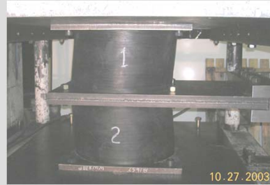
LEAD RUBBER BEARING WEAR TESTING AT VELOCITY OF 3mm/sec, LOAD=2000kN 16,000 CYCLES, TOTAL TRAVEL 1600m
